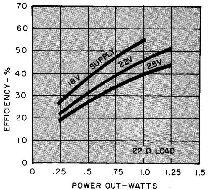
Figure 4. Typical Efficiency vs. Power Out
