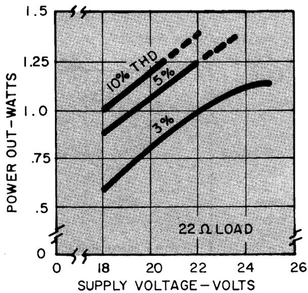
Figure 3. Typical Power Output vs. Supply Voltage
