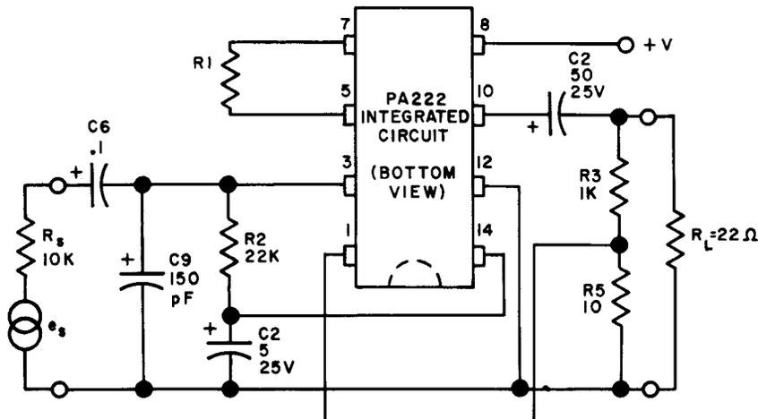
Figure 7. Extended Frequency Range Amplifier
